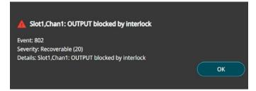
The Operation Status Register provides the interlock's status. The following TSP commands return the status of the interlock.
