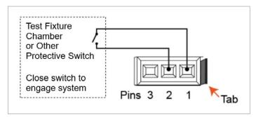
For more information on assembling the interlock, see the MP5103 Modular Precision Test System User's Manual.
